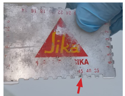
45 MILS WET FILM THICKNESS
